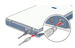
Plug the flat end ♣️♠️♠️ of the cable into any available USB port on your computer.
